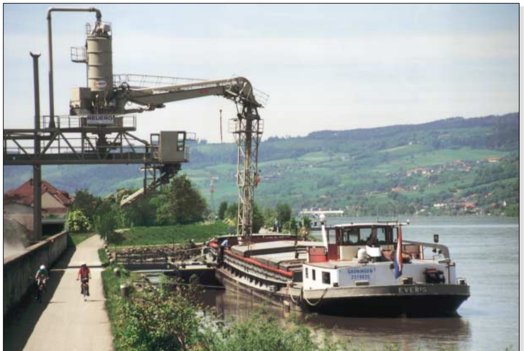
Figure 3 The NEUERO stationary flexiport
